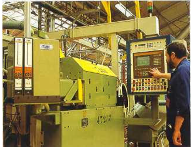
For micron precision, finishing is done using centreless grinding machines.
