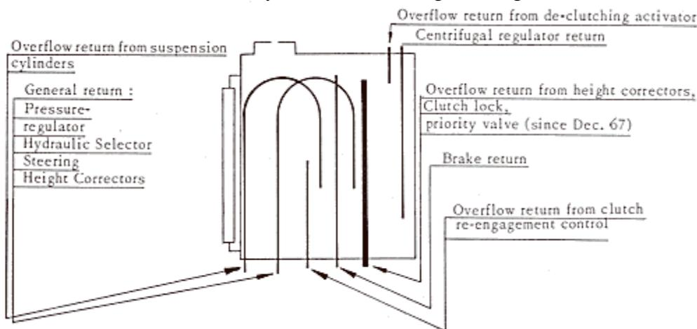
b) Reservoir for vehicles with manual control of gearchange and clutch.
