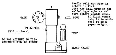
Tester is shipped dry. Open fill plug, and fill as far as possible with fluid. Replace fill plug. Continue filling at "A" to the top of the tester.
