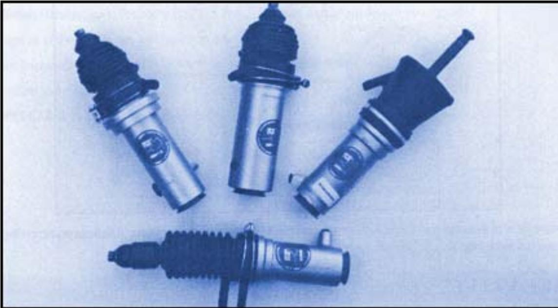
Suspension cylinder failure can be recognised by (A) External Leakage (B) Car sinks rapidly in the affected area. Suspension cylinders are not always suitable for reconditioning due to excessive corrosion.
