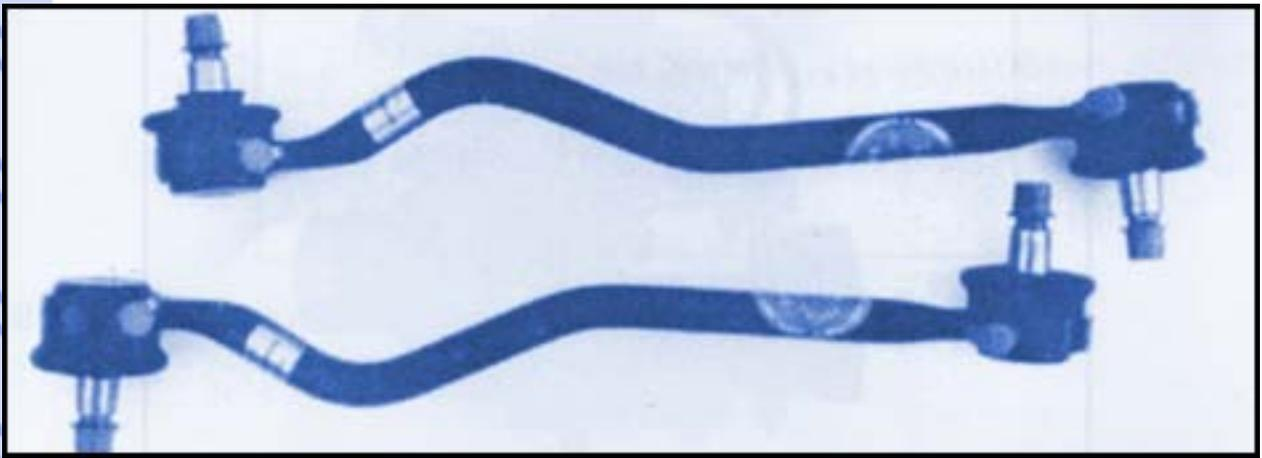
DS or SM track rod failure can be caused by excessive play in the ball joint, resulting in loose steering in extreme cases and MOT failure.
