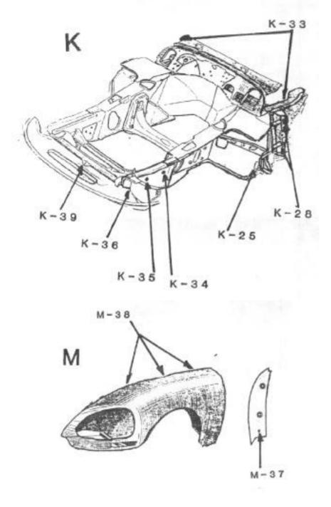
Spray the front fenders (M) through the small hole on the back edge side (M-37) just below the lower rubber horn mount. Spray inside the fender to get some oil where the inner fender meets the outside fender (M-38). This is a very bad place for rust once the fender liner splits and starts to pull away from the outer fender.
