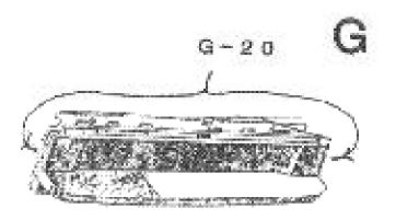
Now, it is time to move onto the tailgate (G) Drill two holes on each side at (G-20), oil and plug up. Move up to the hatch (H). Pull the four rubber plugs out (H-21), oil and return the plugs. Now, lightly spray oil on the outside of the car below the side windows where the body meets the inner fender liner (1-22). This area is prone to separation from the body causing moisture entrapment and rust. Keep an eye on it!
