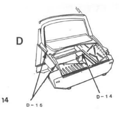
place on the back section of the car that you want to keep lightly oiled, especially if you are going to keep the car parked outside, is the area by the trunk hinges and rain gutter. (D-15) is an area that gets punky on cars, and often a nasty putty job can be found here when looking at that previously owned car.
