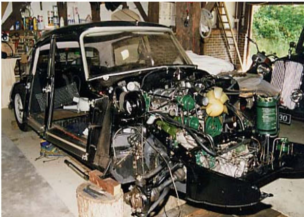
The engine gearbox assembly back in the restored chassis and ancillaries plus hydraulic units being re-fitted. Note that the car is supported each side by two tree trunks under the re-inforcing point. Underneath the car is a full length pit, which makes fitting things like the exhaust system so much easier. In the background is my 1946 Rover P2 14hp.
