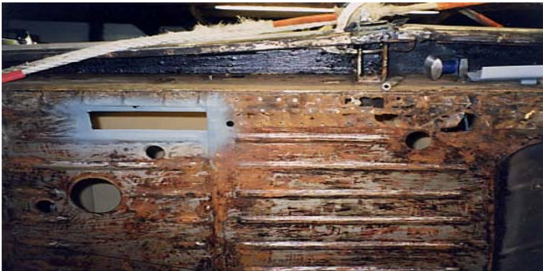
The corroded floor pan. Rusted parts were cut out and dealt with in sections. By welding in new metal in lengths of not more than a foot long, panel distortion was avoided. After cutting out the rust, the panel edges were primed with a Zinc rich weld-through primer, before new 18 gauge metal was Mig welded in. At the top of the picture you can just see the white tow rope to which the engine crane was attached.
