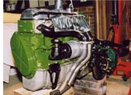
The restored engine waiting to go back in the car. The twin exhaust downpipes are now stainless steel; as are most fasteners used throughout the restoration.
