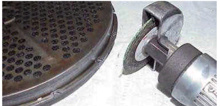
Fig. 4 : But with a grinder, removing the welds is no problem
