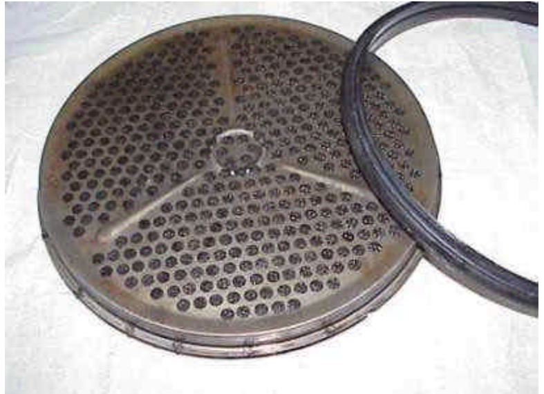
Fig. 2 : First remove the rubber ring.
