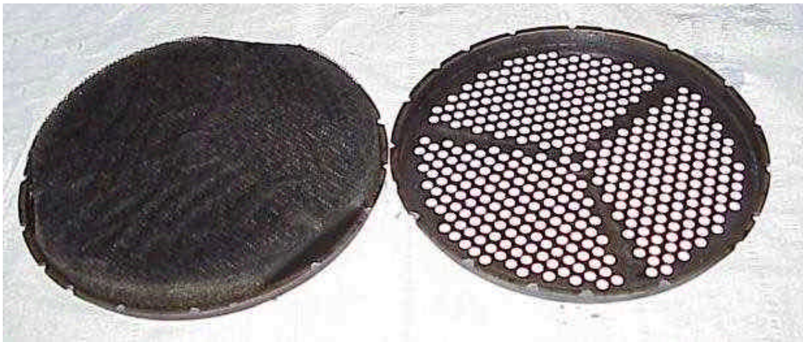
Fig. 5 : When all the welds are removed with the grinder, one can open the filter
