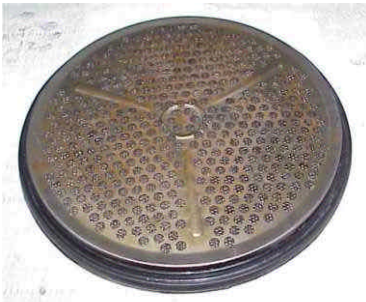
.Fig. 6 : The inside of the filter unit consists of a pile of meshed wire discs.
