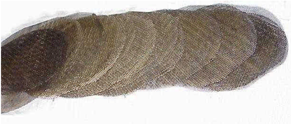
.Fig. 6 : The inside of the filter unit consists of a pile of meshed wire discs.
