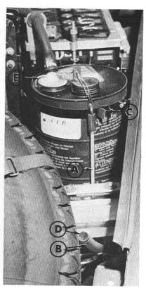
To achieve this start the engine, accelerating slightly to save time. Set the lever **A** (fig. 23 and 24) to position 5 and wait until the car has settled at its maximum height.
