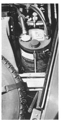
The oil level must reach the upper "High" notch of the dipstick without exceeding it.
