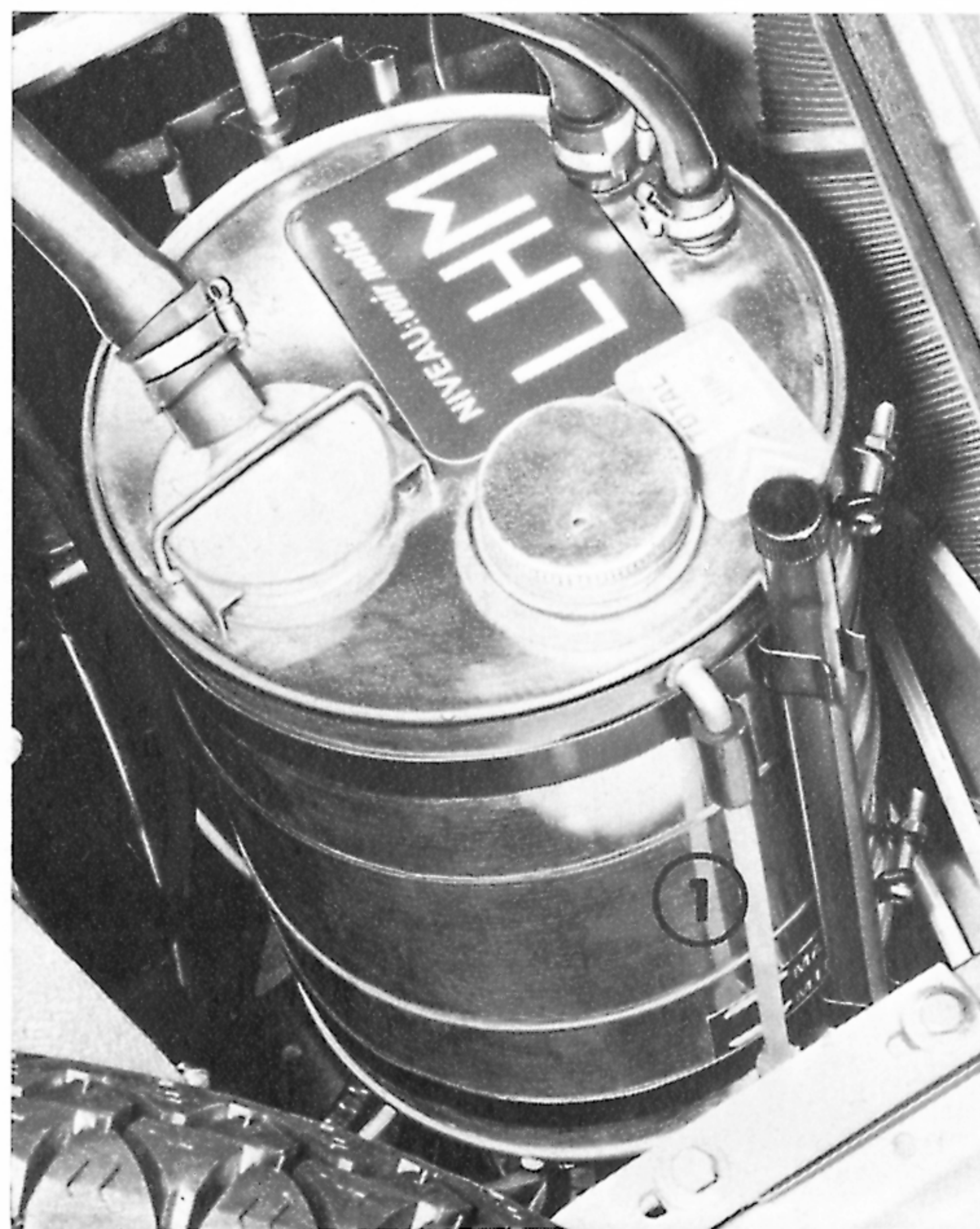
Fig. 26 - Hydraulic reservoir 1 - Level checking sight-tube
