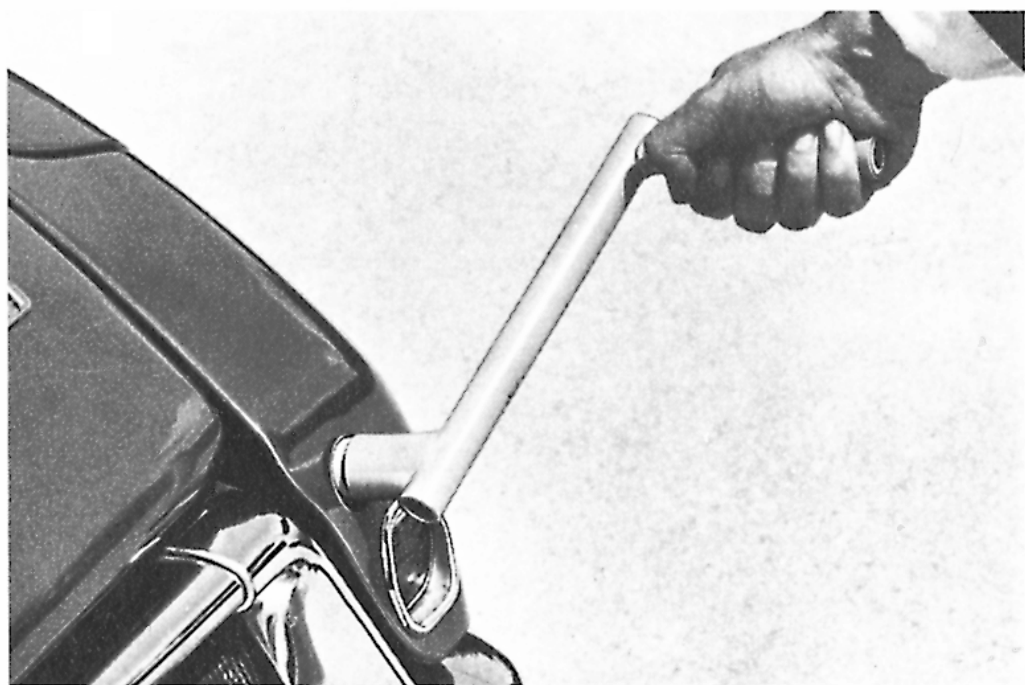
Fig. 32 - Removal of a rear wing
