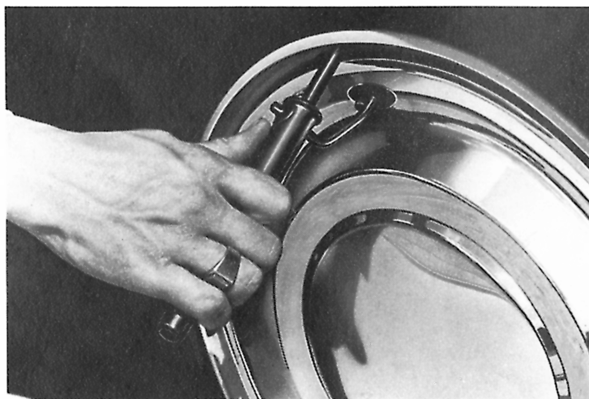
Fig. 33 - Removing wheel embellisher
