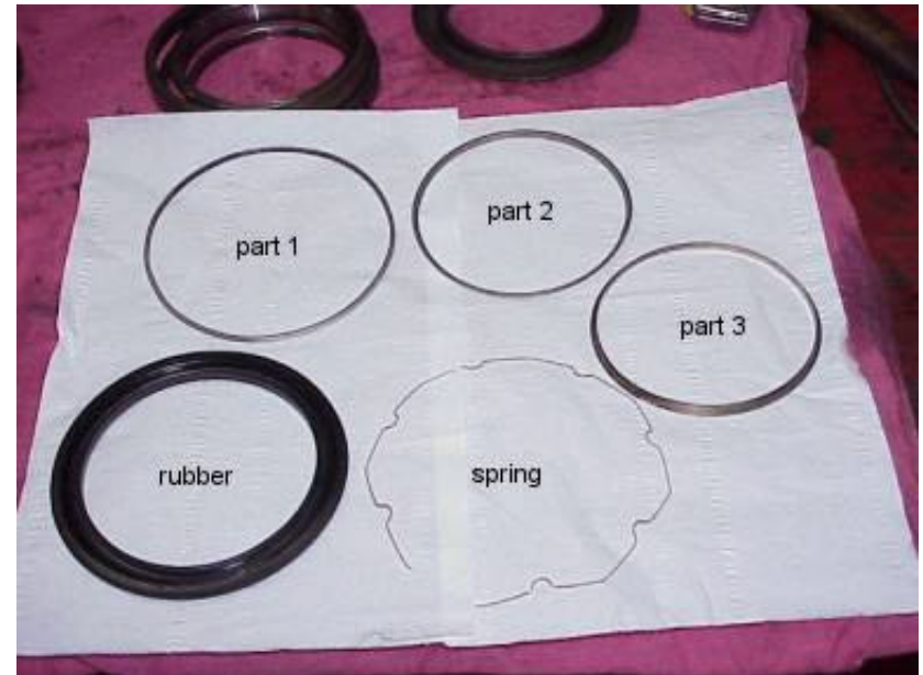
Fig.2 : All the parts that form the seal
