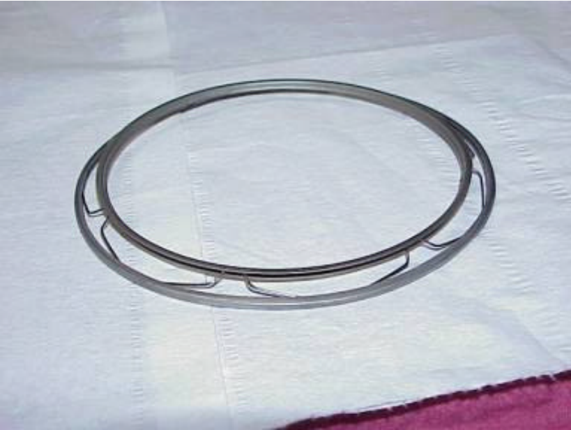
Fig.7 : Framework (metal parts 1 and 2 + spring)
