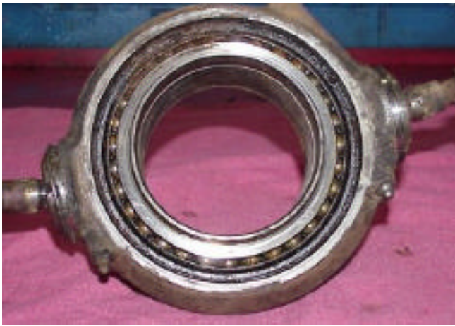
Fig. 8 : Grease seal removed
