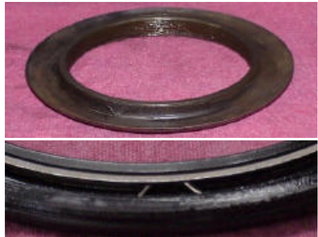
Fig. 6,7 : Underside of the ring nut, detail of grease seal
