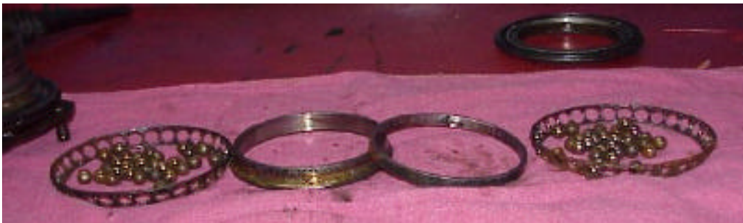
Fig.12 From left to right : a bearing separator, a race, the spacer and the other separator together with some balls.
