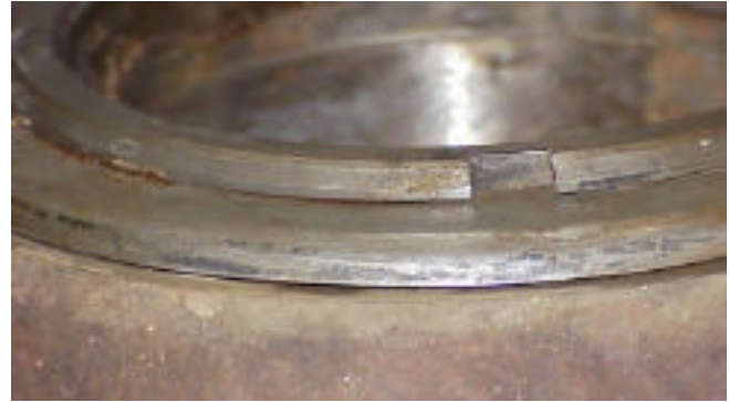
Fig. 4 : Detail of ring nut with notch and shield
