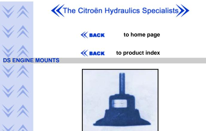
DS engine rubber mountings damp out the vibrations of the engine to the car body. Failure of the rubber can be indicated by the increased vibration in the car which is engine speed related.
