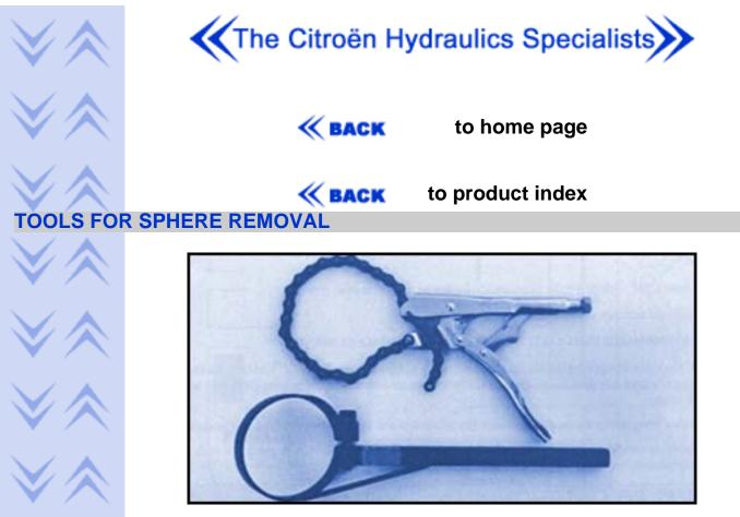
Our band wrench has been specifically designed to remove all spheres (except split type).
