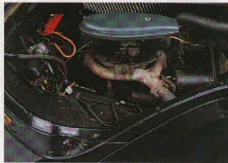
Engine is robust but water pumps can leak
